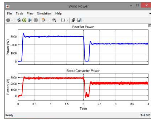
Figure 5. Wind turbine power output based Neural Network
