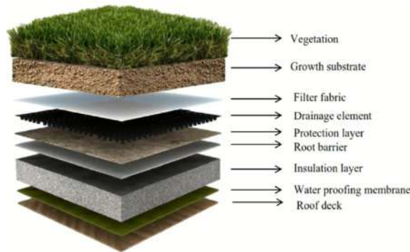
Figure 1. Layers of a Green Roof Simulation [5]
