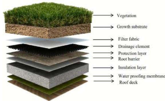
Figure 1. Layers of a Green Roof Simulation [5]
